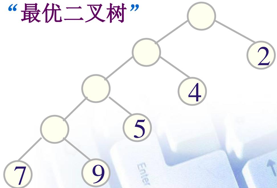
$$\begin{aligned} \text{WPL}(T) &= 7 \times 4 + 9 \times 4 + 5 \times 3 \\ &\quad + 4 \times 2 + 2 \times 1 = 89 \end{aligned}$$
