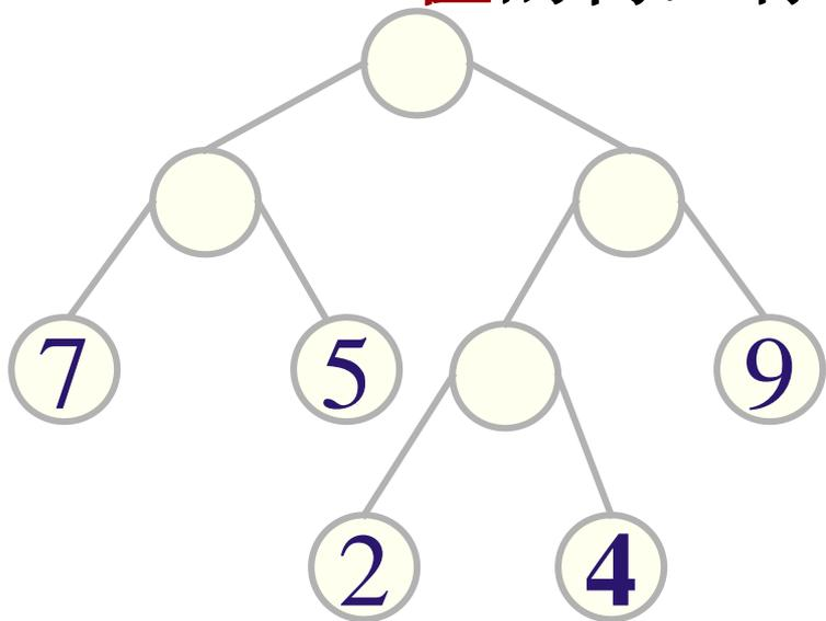
$$\begin{aligned} \text{WPL}(T) &= 7 \times 2 + 5 \times 2 + 2 \times 3 \\ &\quad + 4 \times 3 + 9 \times 2 = 60 \end{aligned}$$
