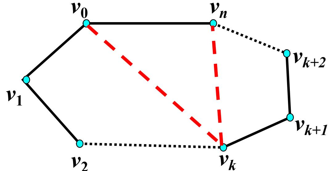
$$T_P = T(v_0, \dots, v_k) \cup T(v_k, \dots, v_n) \cup \{v_0 v_k v_n\}$$
